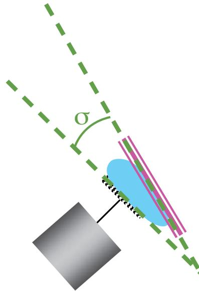
This causes the laser beam to trace out an oval shape. The size and the shape of the oval depends on the angle  $\sigma$ . All of this oval shape needs to land onto the second rotating mirror. The mirrors are quite small so need to ensure that  $\sigma$  is quite small and that the two mirrors are close together. The motors can be held by clamp stands or if you are feeling adventurous you can build your own stands.
